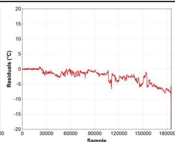
Figure 7. Residuals  $T_{C,o}$ , period after the first heat exchanger cleaning
