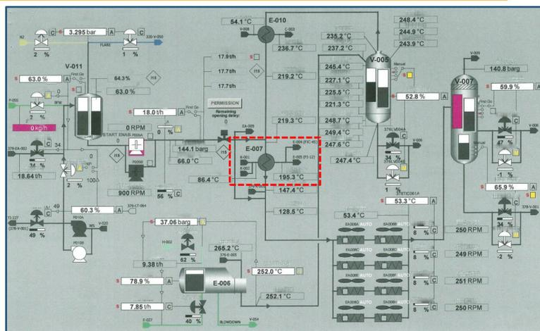
Figure 1. Hydrocracker unit with E-007 heat exchanger
