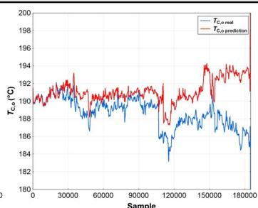
Figure 6. Comparison of actual and predicted  $T_{C,o}$ , period after the heat exchanger cleaning
